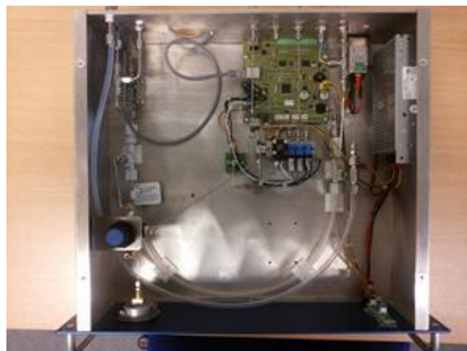
Sample conditioning unit with Perma Pure dryer and humidity sensor
